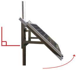
6. Lift the bottom of the Solar Panel until the attached arms holding it are angled at 90 degrees. Tighten all 6 bolts again from and face the panel north.
